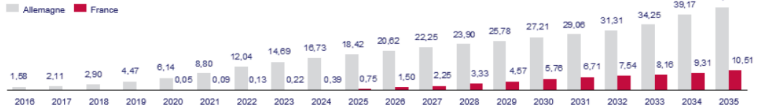
EVOLUTION OF THE WIND FARMS THAT NEED TO BE DISMANTLED (CUMULATED GW)
